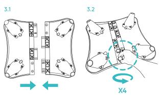
Connect the table plates together using 4 bolts.
