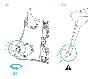
Screw the table legs into the holes on the underside of the table.
